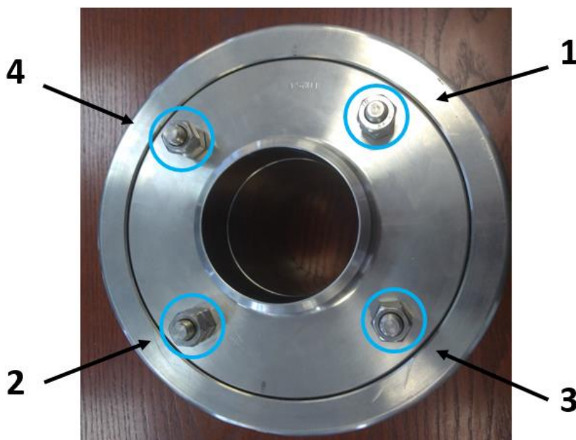
Figure 15: Preload Torque Application
