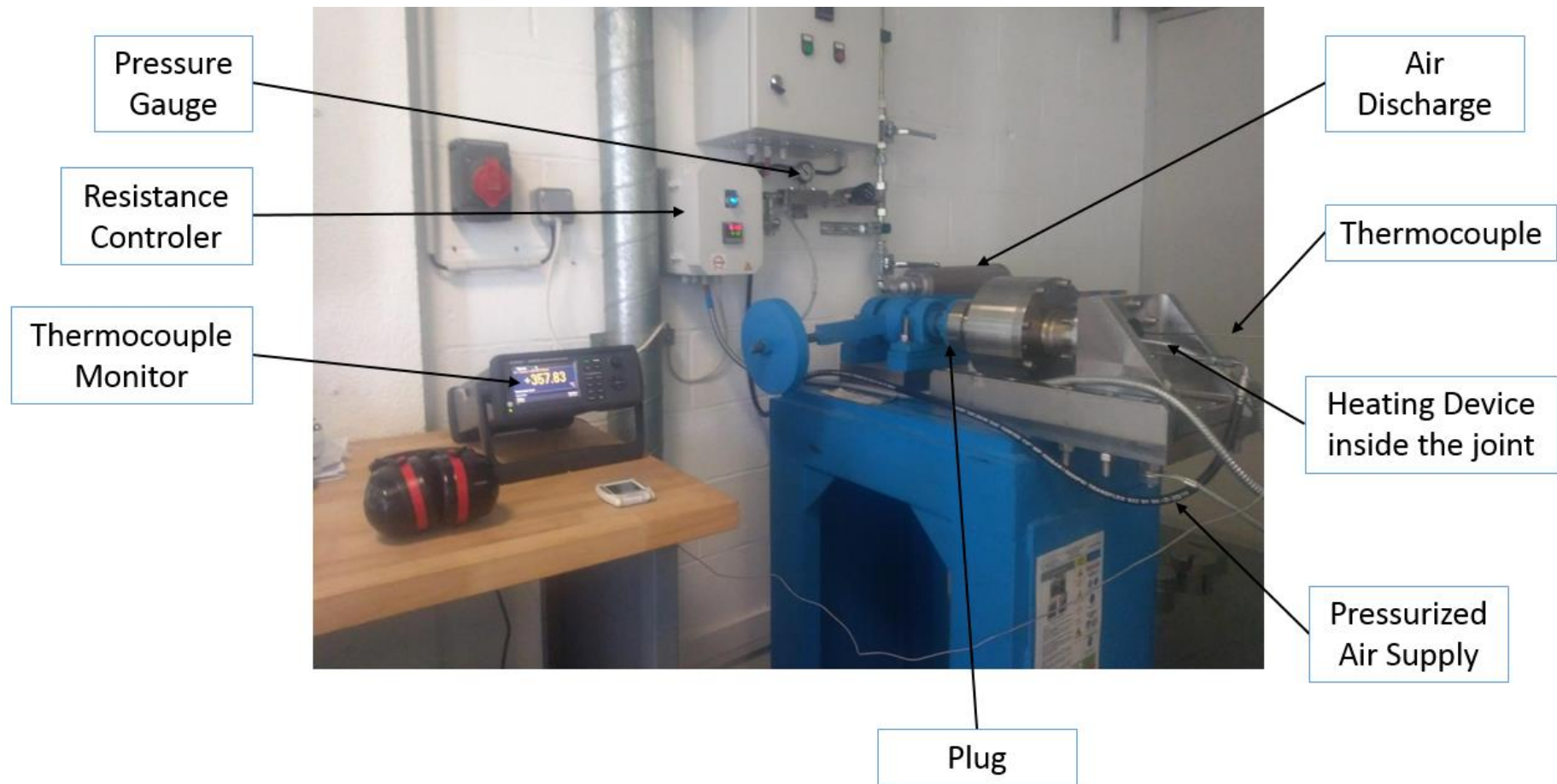
Figure 9: Leakage Test Bench
