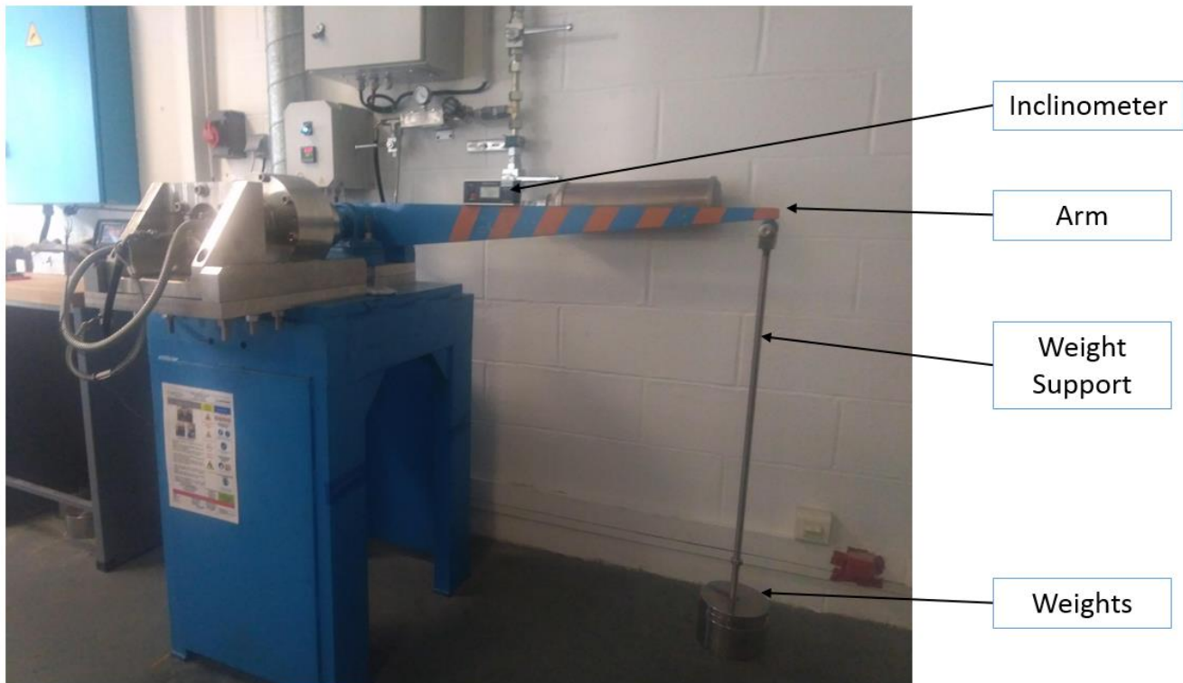
Figure 12: Angular Stiffnesses Test Setup
