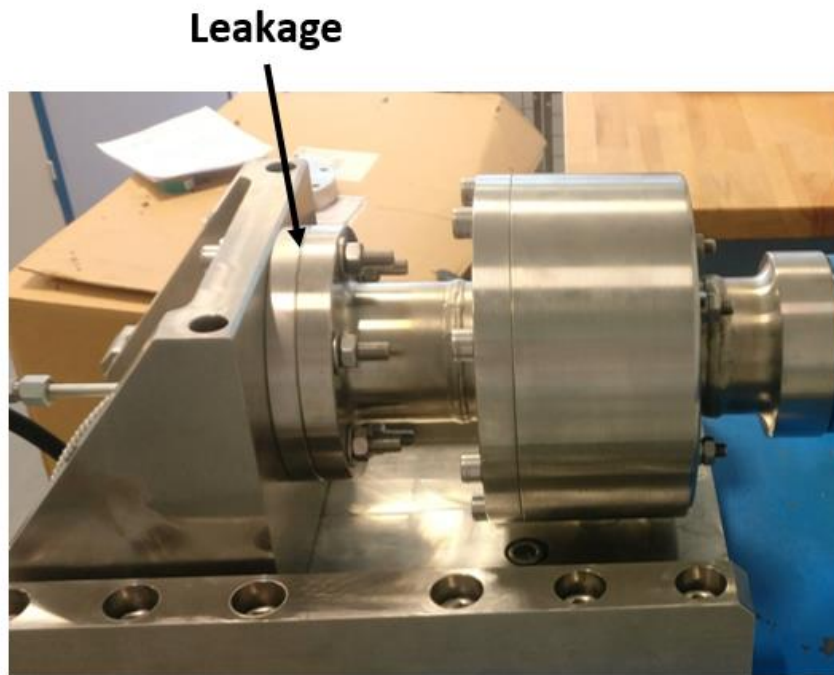
Figure 13: Location of the leakage on SDU side
