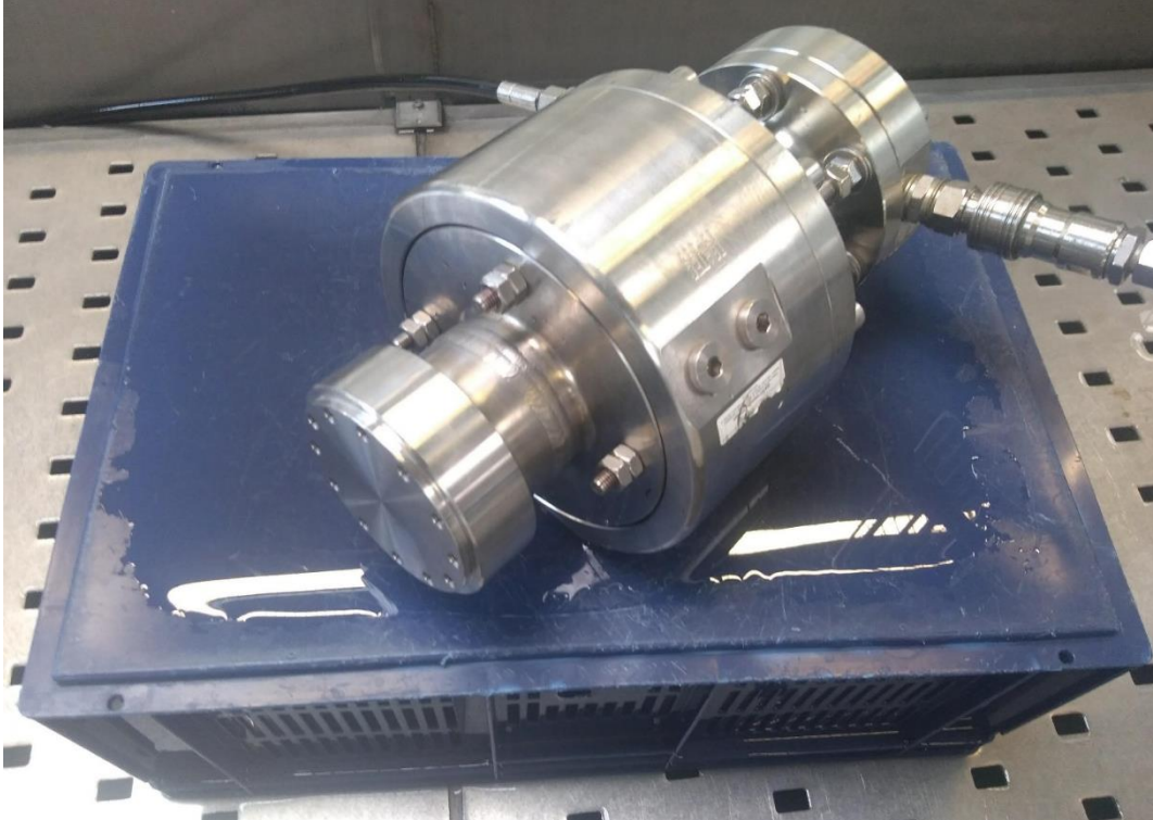
Figure 6: View of the Swivel Joint during Proof Pressure Test
