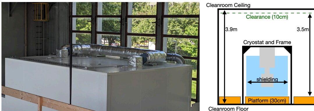
Figure 3 : Left: Photograph of the trap on top of the clean room. The size of the trap door is 2 m x 2 m. The maximum height of the parts that can be lifted by the crane from outside the clean room to inside, via this trap door, is about 1.5 - 1.6 m. Alternatively, parts can be brought inside the experimental area via its direct access door of 1.8 m width and 2 m height. Right: sketch showing the room and platform dimensions.
