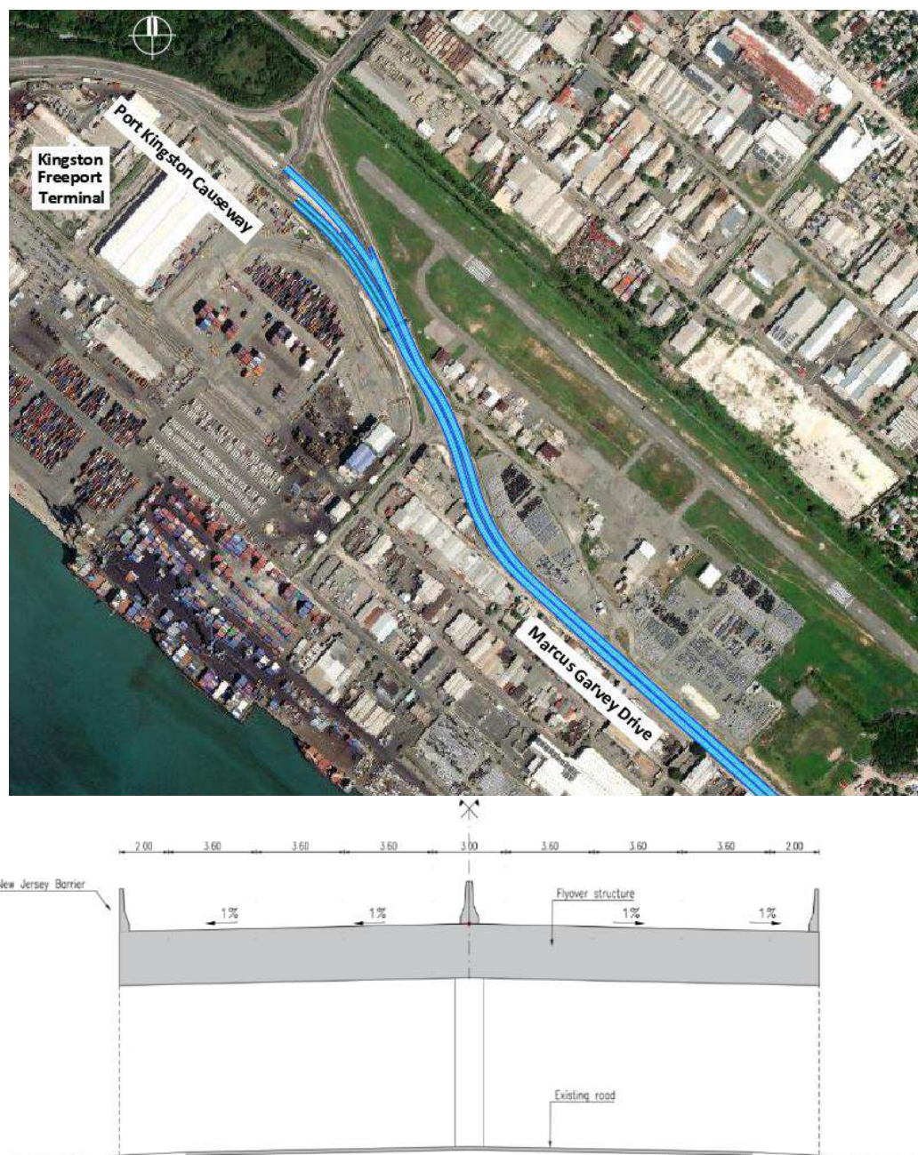
Figure 17: Proposed alignment of the elevated roadway option and cross section of the proposed roadway.
