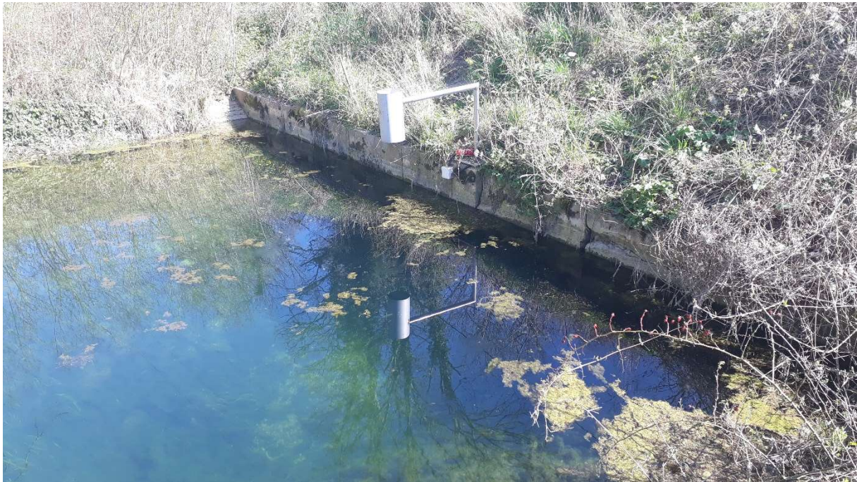
Figure 6 : Sonde radar aval.
