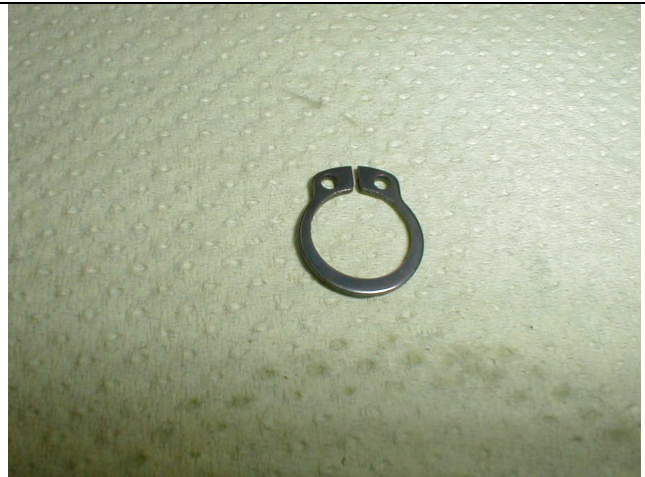
The large actuators are locked with Seeger ring.
