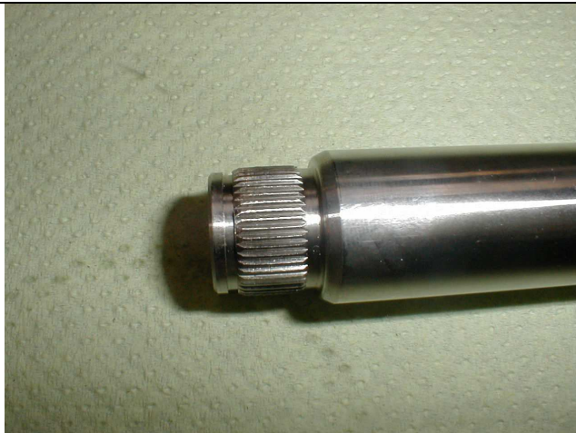
New spline connection.
