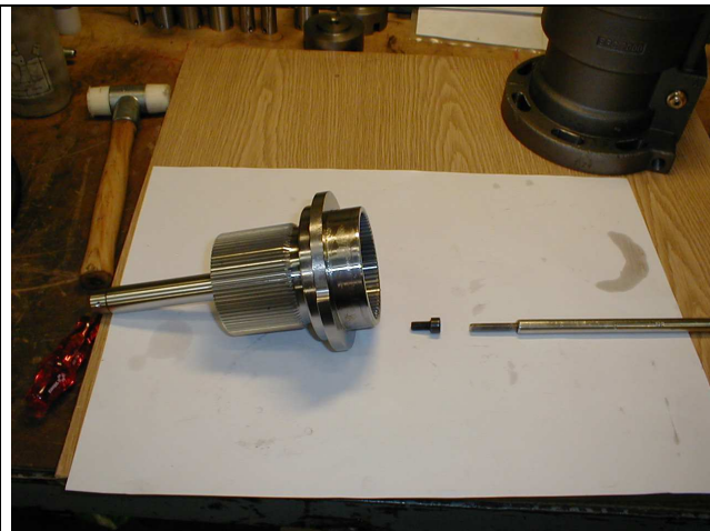
The spline shaft is dismounted.
