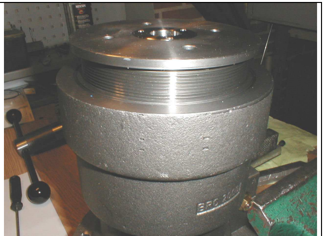
The top part is dismounted. Use special tools or 2 pins fitting the holes in the top part. Note: Turn clockwise to loosen the top part.
