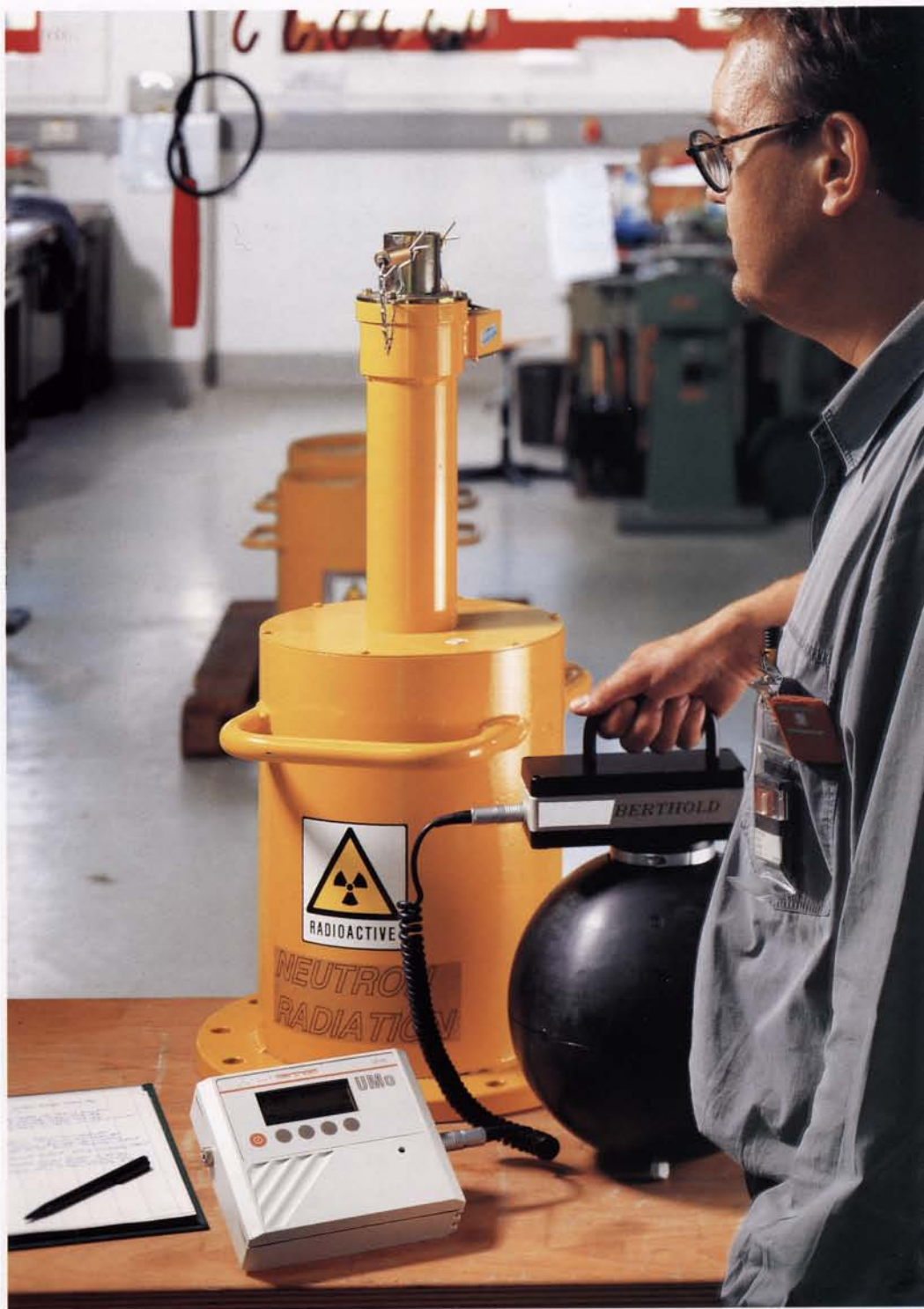
LB 6411 neutron probe as portable monitor used for measuring the neutron dose rate on an industrial Am-Be-source for moisture determination.
