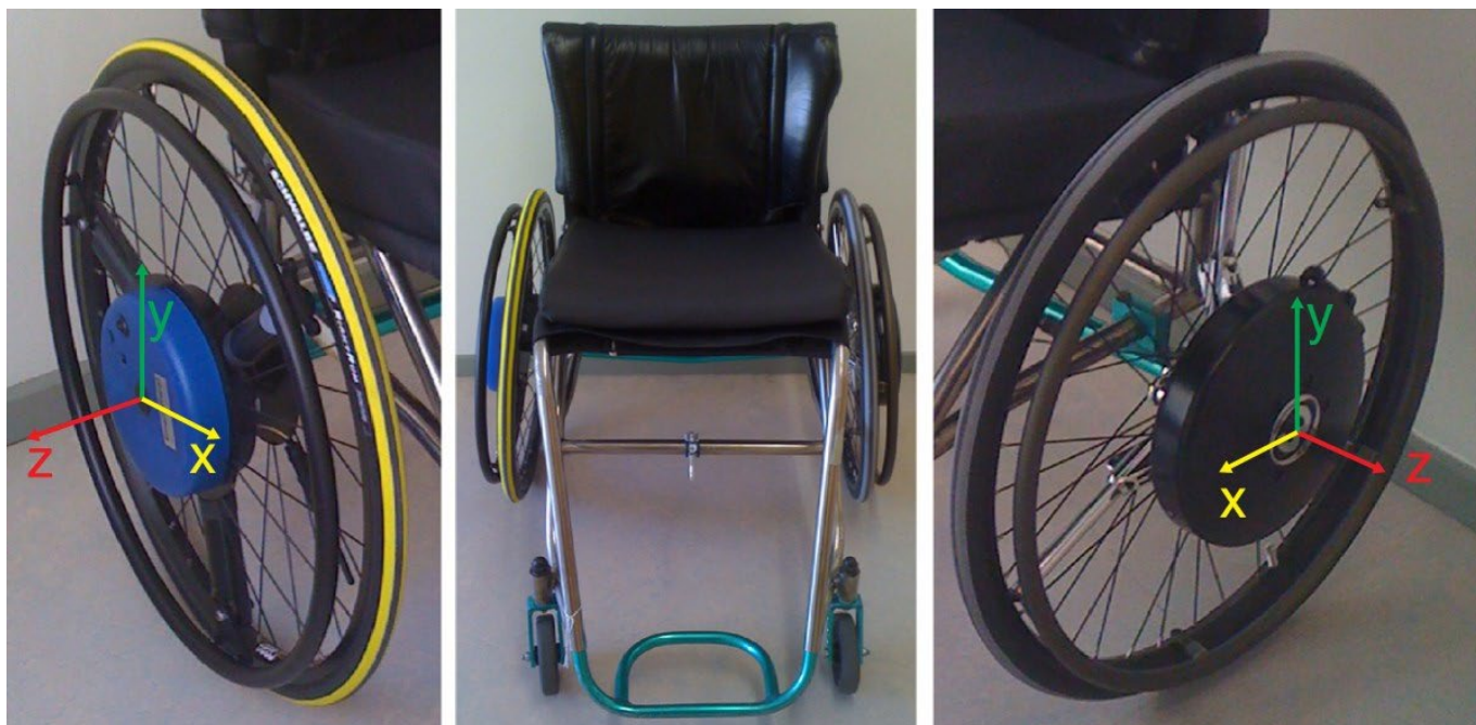
FIGURE 1: ILLUSTRATION D'UNE ROUE À MAIN COURANTE INSTRUMENTÉE ISSUE DE LA PUBLICATION "VARIABILITY IN BIMANUAL WHEELCHAIR PROPULSION: CONSISTENCY OF TWO INSTRUMENTED WHEELS DURING HANDRIM WHEELCHAIR PROPULSION ON A MOTOR DRIVEN TREADMILL" VETGER ET AL., 2013
