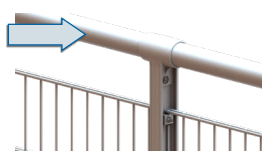
Rupture main courante
